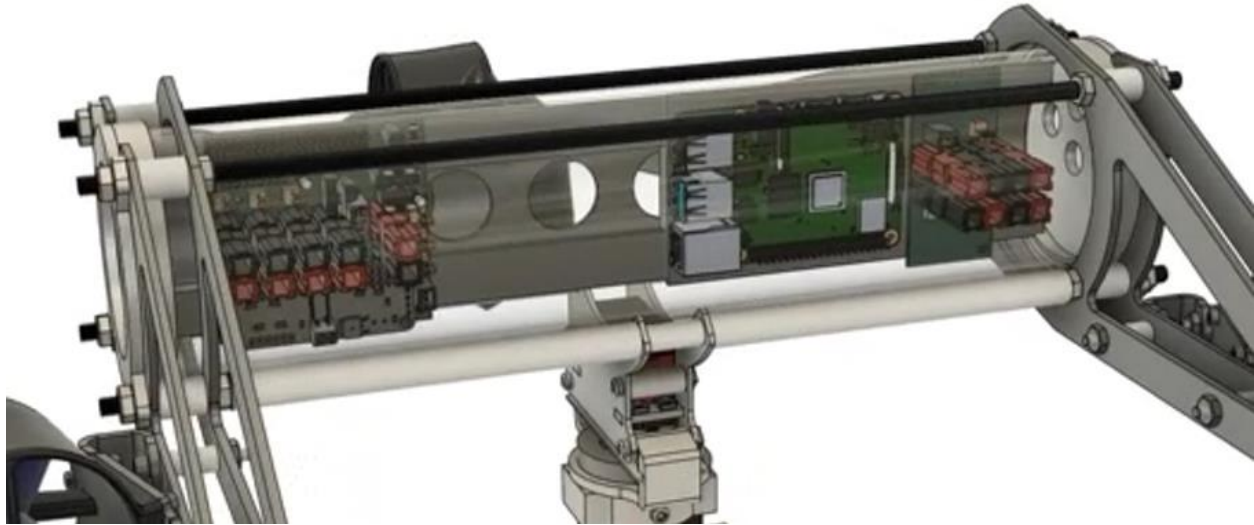
Figure 16 : Mechanical Integration of the PCBs
