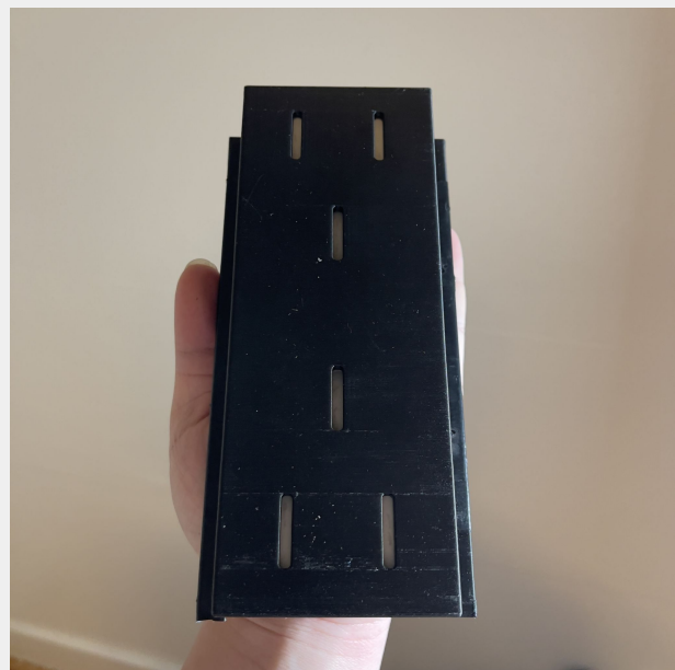
(Fig. 27) Holes at the bottom of the ballast container to create a water drain
