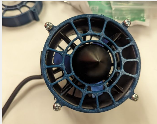
(Fig. 22) T200 thruster with custom 3D printer shroud
