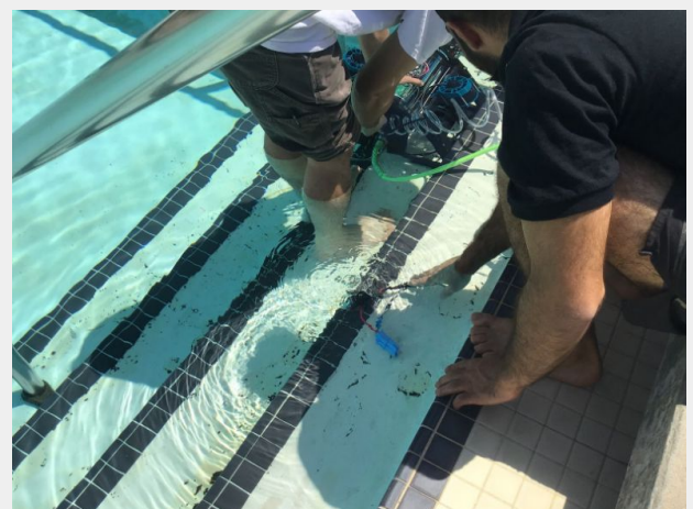
(Fig. 41) Air escaping from main canister through the top-side end of the ethernet cable.
