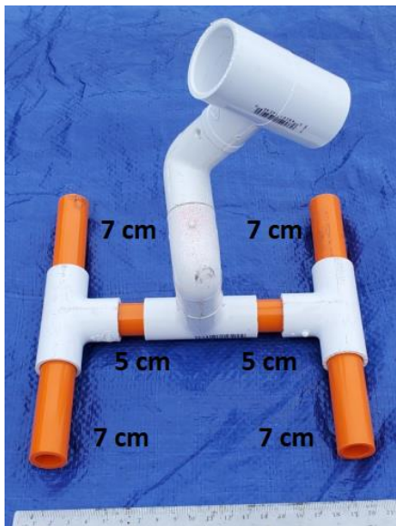
Left: Acoustic receiver front view constructed from 1/2-inch PVC pipe. Right: Acoustic receiver side view.
