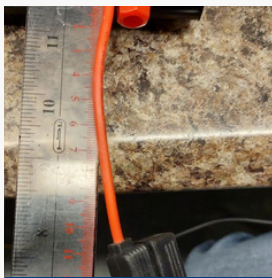
Figure 23: Fuse ~10.5cm from power supply Credit: Waffa Zahralyn
