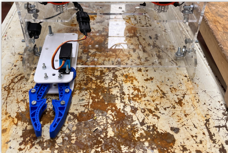
New skid with manipulator
