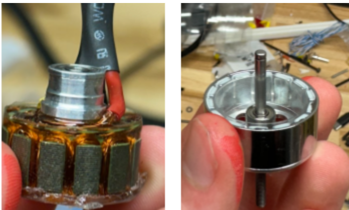
Fig. 14 (a) An image depicting the rotor and copper wiring of the brushless motor coated in epoxy. (b) The stator shown, coated in epoxy.
