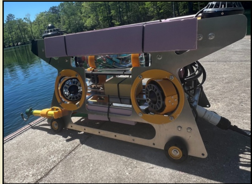
Figure 12. Second iteration of buoyancy testing with 250 Extruded Polystyrene- XPS.
