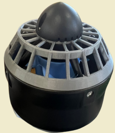
Figure 16. 3D-printed shrouds are used to protect wildlife and operators from thruster motion.
