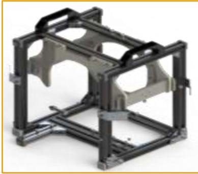
Figure 9: Kratos ROV's main frame structure CAD design by solidworks
