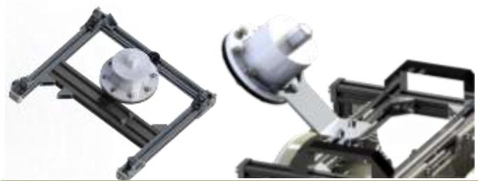
Figure 15: (Left) Bottom camera mounting by Solidworks & (Right) Back vision camera and L shaped Aluminum Fixation.
