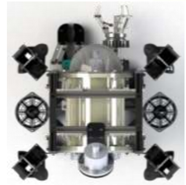
Figure 18: Kratos ROV's top view of thruster configuration by Solidworks.
