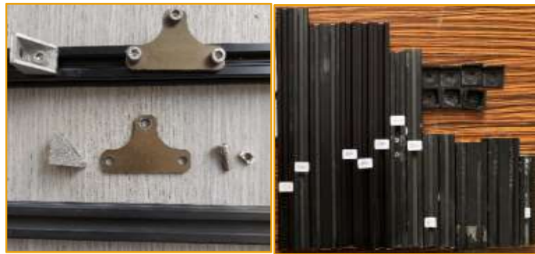
Figure 10: Al-extrusion and its accessories captured by Hoor.
