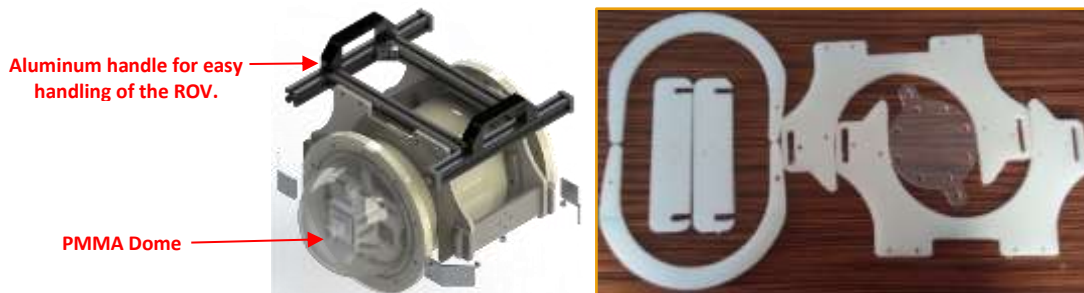
Figure 11: (Left) Enclosure and its holder CAD parts by Solidworks & (Right) Manufactured parts of the enclosure holders.
