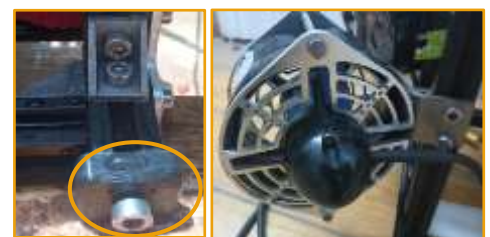
Figure 13: (Left) 3D printed part Thruster & (Right) sheet metal bent L mounting captured
