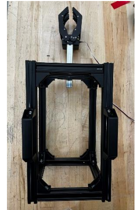
Figure 10: Aluminum ROV frame with claw.
