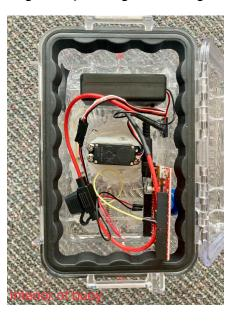
communication with the receiver. The receiver can be turned on and off via a switch on the outside. When the buoy is at the surface the LCD should display the time and team number.
