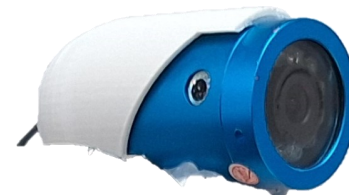
Infra-red Nav Camera Photo Credit: N Scott
