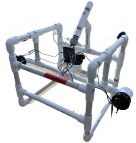
Figure 5: The Great White 1 frame structure
