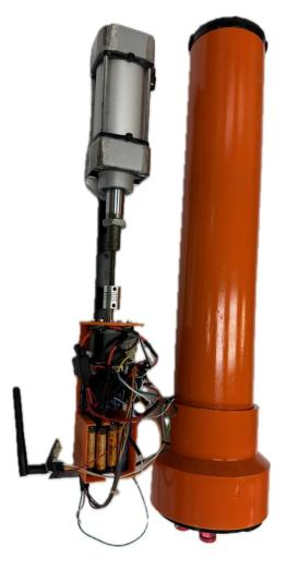
When at the surface, the Remora will communicate with the mission station using two paired transceivers, one within the Remora and the other within the surface receiver box. The transceiver is capable of interfacing with Arduino, which information allows for the communicated to be easily modified. When the information is communicated with the mission station, an Arduino Uno reads it and sends it to the laptop to be graphed.
