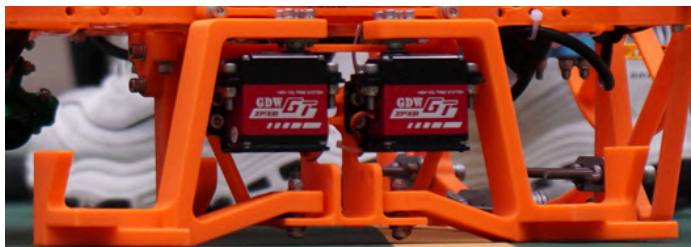
Figure 9. The Installed Gripper
