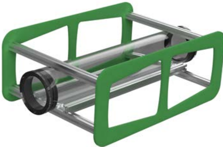
Figure 2: CAD Model of STEVE ROV Frame
