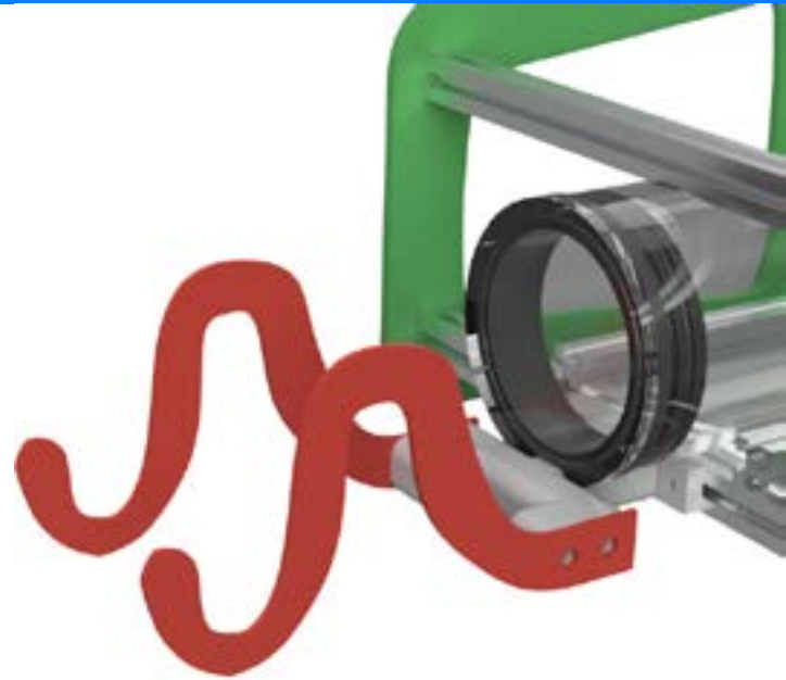
Figure 5: CAD Model of STEVE ROV Manipulator
