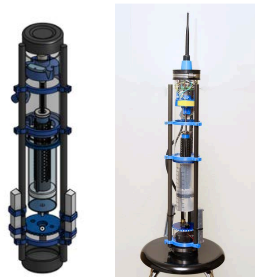
Figure 36. CAD and Completed Float
