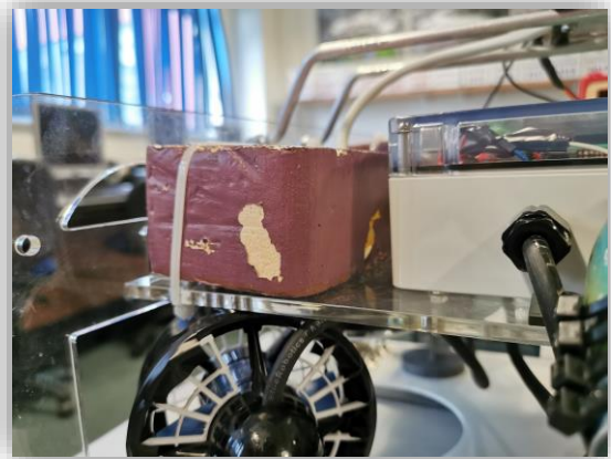
Buoyancy block - Photo by Lewis Smith
