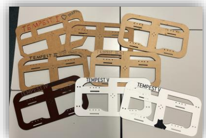
The evolution of side plates for Tempest I to V - Photo by Eilidh Payne
