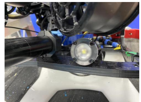
Fig. 14 LED lights mounted on the middle layer
