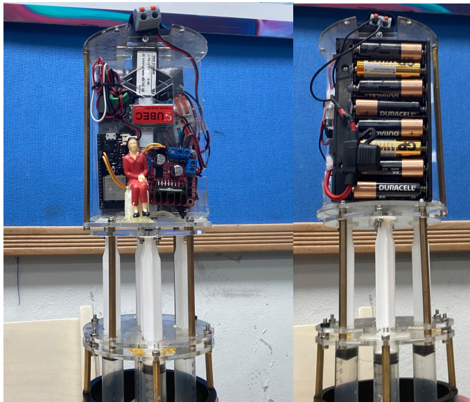
Fig. 1 Interior of the vertical profiling float
