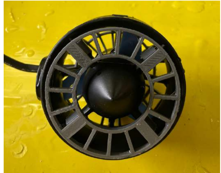
Figure 13. 3D-printed shrouds are used to protect wildlife and operators from thruster motion.
