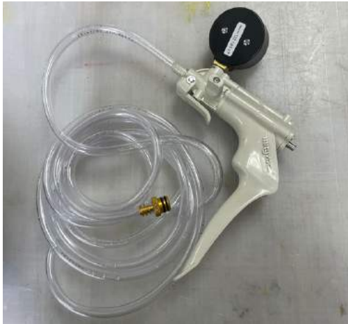
Figure 5. A vacuum pump used to pressure test the Blue Robotics electronics enclosure.
