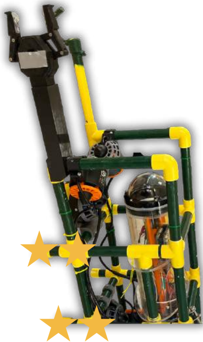
Figure 18. The stars represent the final placement of lead weights within the PVC frame.
