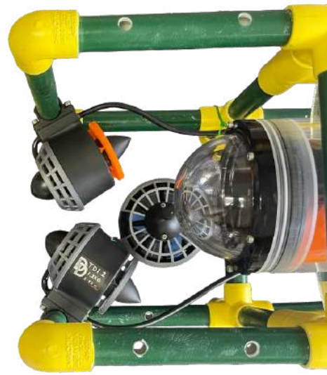
Figure 6. One vertical T200 thruster and two horizontal (and angled) Diamond Dynamics thrusters.
