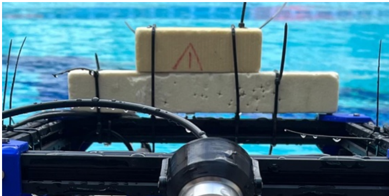
Fig. 19 - Foam blocks reused to counteract the weight of the tether
