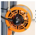
Customized motor shrouds to ensure safety to objects in and out of the water. Orange fill was used to make workers aware of the motor's location.
