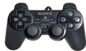
Fig 3.16 PS2 gamepad for controlling of ROV.
