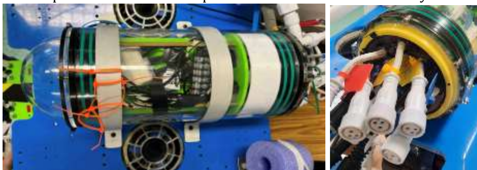
Fig 3.21 ROV waterproof cylindrical closure (Photo by Javen)
