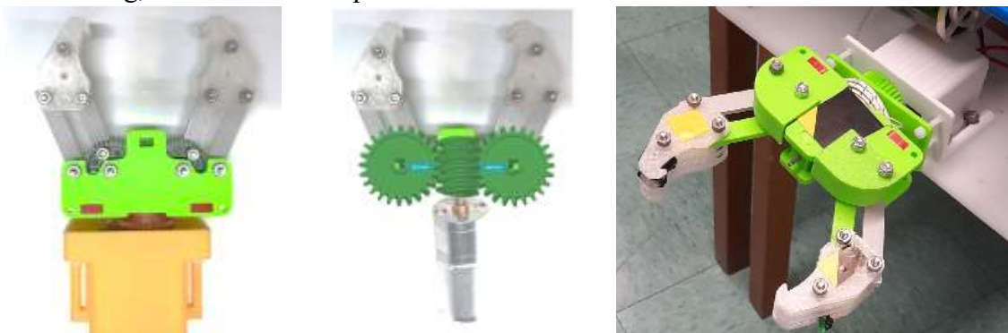
Fig 3.13 3D design of the payload with worm gear system (Photo Credit: Cheung)
