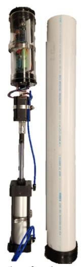
When at the surface, the Barnacle will communicate with the mission station using two paired transmitters, one within the Barnacle and the other within the surface control box. The transmitter is capable of interfacing with Arduino, which allows for the information communicated to be easily modified. When the information is communicated with the mission station, another Arduino Uno reads it and then displays it on an LCD screen.
