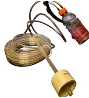
Figure 15: eDNA extraction Device
