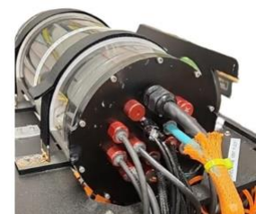
Figure 27 : All penetrators are waterproofed with epoxy
