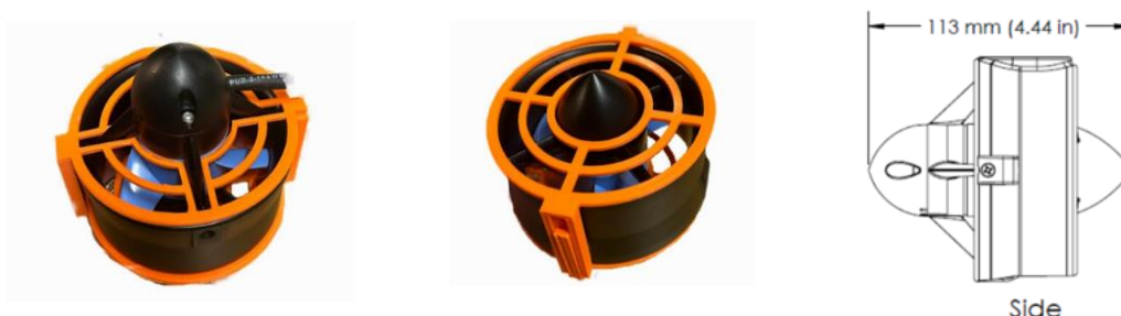
Figure 6: T200 Front and Back view of thrusters with custom shrouds and measurements.
