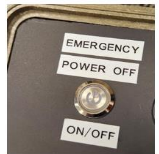
Figure 24: Emergency shut off switch
