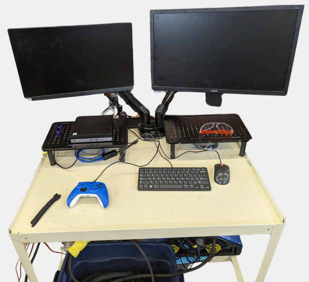
Figure. 12 UR2 built a control station this year rather than developing a control box. With Stingy being an attached to a control box, UR2 can pack the ROV into a traveling case and pack all the surface controls with it.
