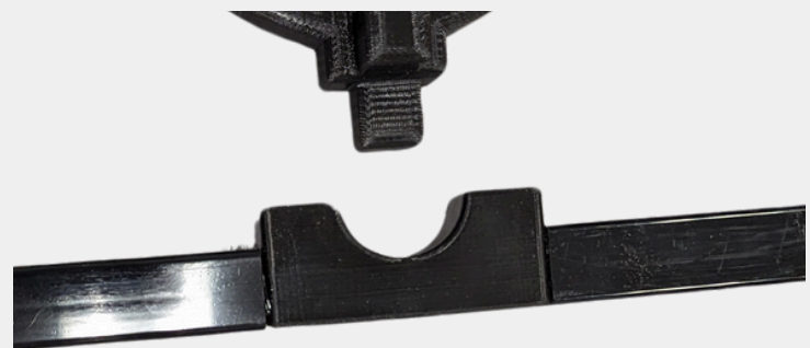
Image: Frame connection part with built-in gripper placement. G Wirgau
