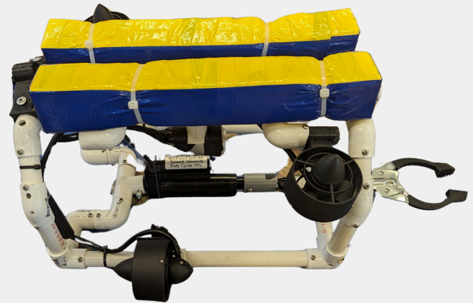
Figure 23. After finishing the dragster project, we moved on to prototyping an ROV powered by four U2 Minis. The frame was constructed using PVC material. Since UR2 had previously tested the building materials for Stingy's frame, we decided to skip building a new one. To connect the thrusters to the frame, we 3D printed different thruster adapters. It took us three attempts to get it right as the thrusters kept breaking the mounts due to the force.
