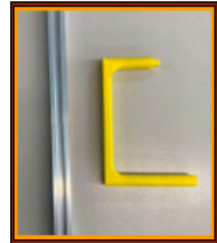
Figure 9: Comparison of metal V-slot rail and 3D printed part.
