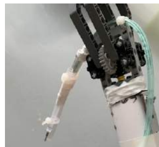
Figure 8 (right): Sample Collection Probe Photo Credits: A. Nasief
