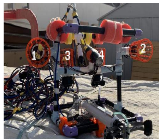
Figure 3: Labelled Motor Placement on the Kraken Slayer
