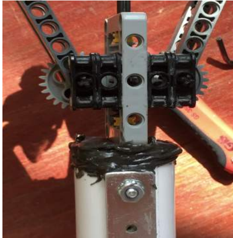
Figure 17: Claw Waterproofing Photo Credits: A. Nasief
