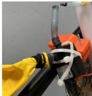
Figure 8 (right): Sample Collection Probe Photo Credits: A. Nasief
