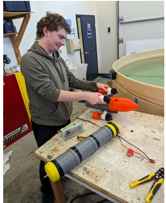
(Above) Clayton, one of our two seniors on the team is testing our 3D printed float prototype. We worked on several prototypes using both TinkerCAD and OnShape to develop our ideas and to 3d print them.
