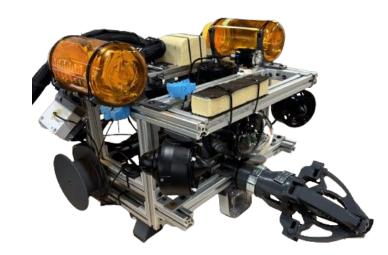
SAFETY FEATURES: topside control box acrylic cover, single shutoff switch, thruster guards, pressure relief valve, pressure regulator
