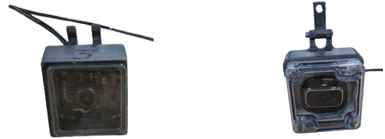
Figure 8: Comparison of original (left) vs. updated (right) camera enclosures - Makenna Reilly
