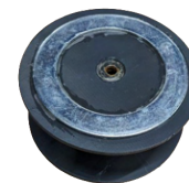
Figure 17: 3D printed spool with inlaid magnet and ring shim - Makenna Reilly
