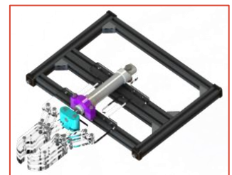
Figure 15: Thruster and bent L mounting by solidworks
