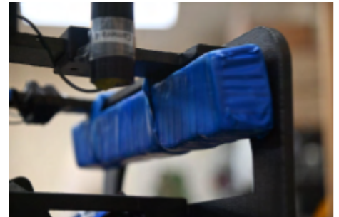
Figure 8: LabraShark's HD Foam for buoyancy. Image by Olivia Normore.
