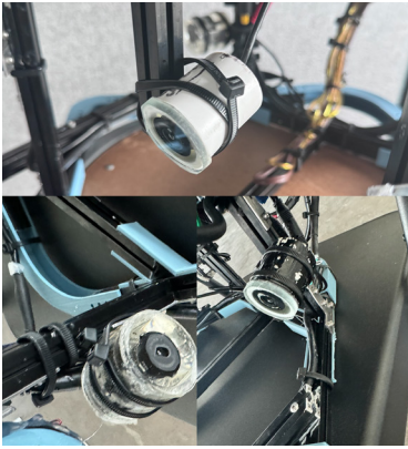
[Figure 20: Claw camera with back left and right below respectively - Photo Credit: Devin Spears]
