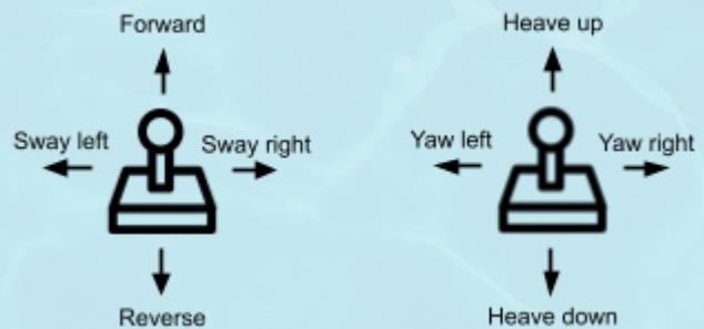
Figure 11: Control stick mapping
