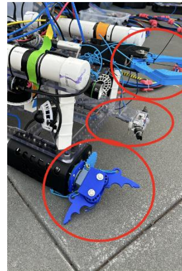
Phase 3 testing of gripper design – float gripper on top, rotating gripper on bottom right and here a fixed gripper in bottom left (later changed to a rotating gripper). Photo: Gust
