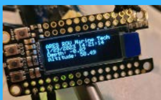
Figure 17: Photo of the data being received and printed by the server.
