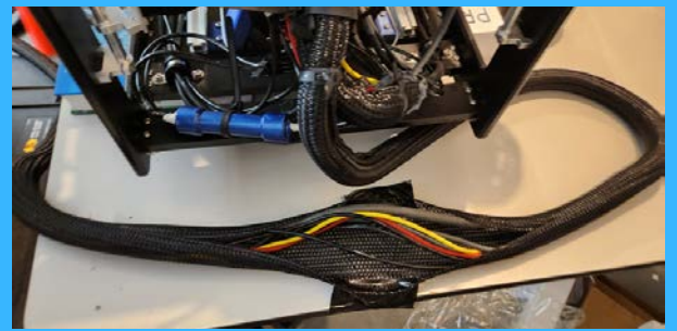
Figure 7: Section of tether showing inner contents.
