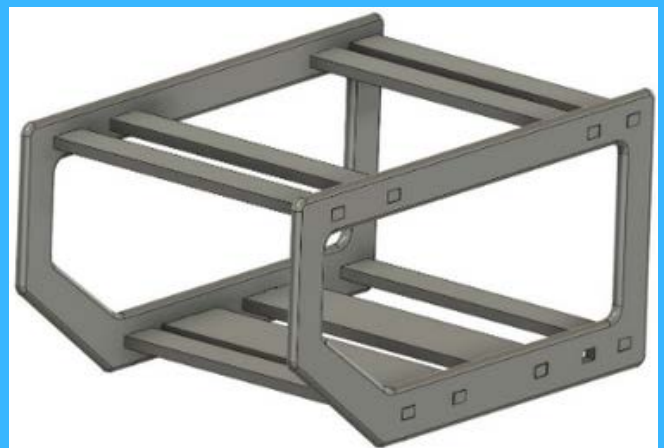
Figure 15: CAD model of custom frame design.
