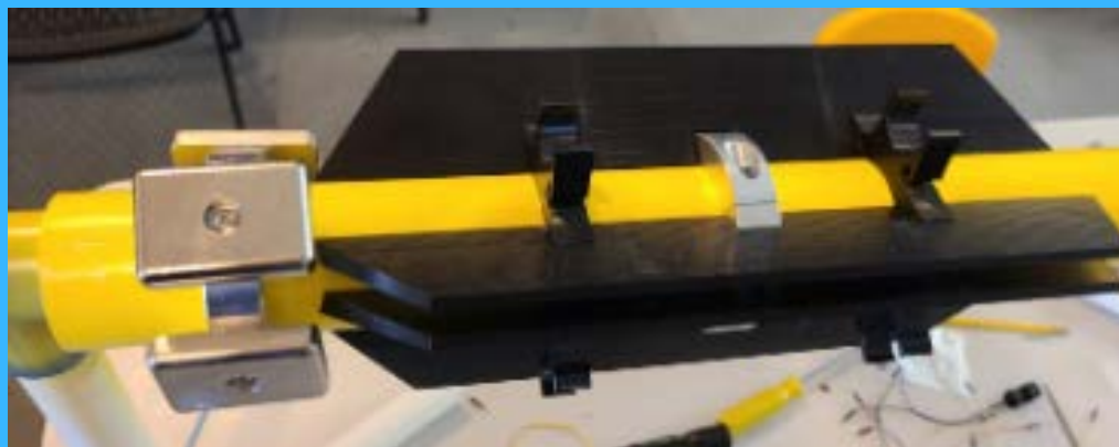
Figure 20: Fins, weight ring, and battery pack clips (without battery packs attached).
