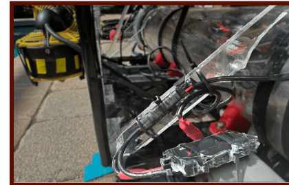
Figure 29: The Temperature Sensor Strapped to PVC
