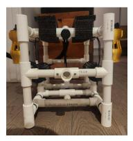
the PVC frame. Screws are put in key locations. We have opted not to use onboard electronics as we are a new team.
