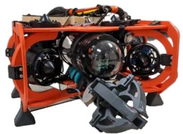
SAFETY FEATURES: topside control box acrylic cover, one shutoff switch, smoothed edges on frame, thruster guards, pressure relief valve, pressure regulator
