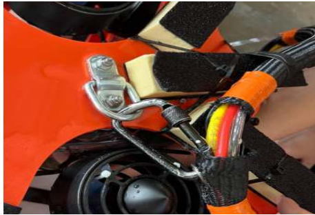
Fig. 15: Strain relief on the robot-side - Violet Brockmann
