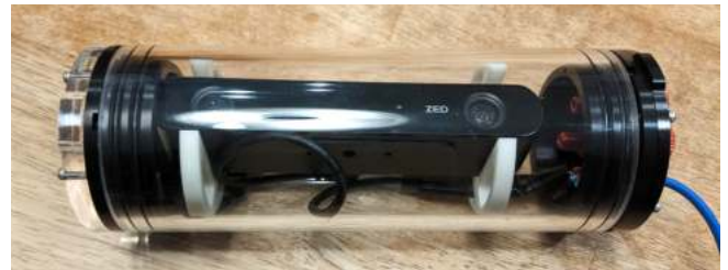
Fig. 25: ZED camera in acrylic tube - Makenna Reilly
