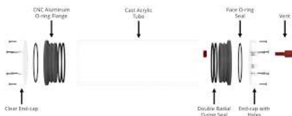
Fig. 7: Electronics housing assembly - Blue Robotics
