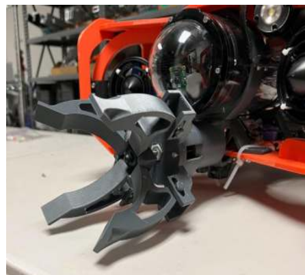
Fig. 22: Claw fully opened - Violet Brockmann
