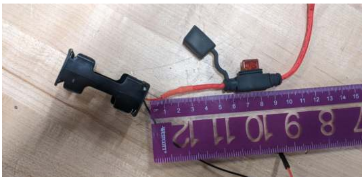
Fig. 2: Fuse within 5 cm of power - Makenna Reilly
