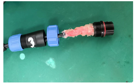
Fig. 14 Camera soldering joint with large heat shrink tube and hot glue
