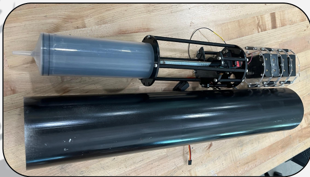
Inside Components of Buoyancy Engine, photo by Isabella Wong.
