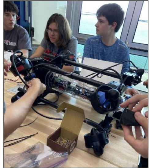
Figure 20: Company members screwing motors into 3D printed joints, photo by Ava Palazzolo.
