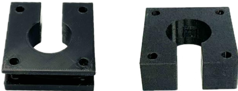
Figures 10, 11, 12 (From left to right): 3D printed motor attachments, photo by Joshua Silversten.
