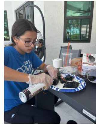
Figure 17: Company CMO waterproofing servos in-house, photo by Maya Venkatesh.
