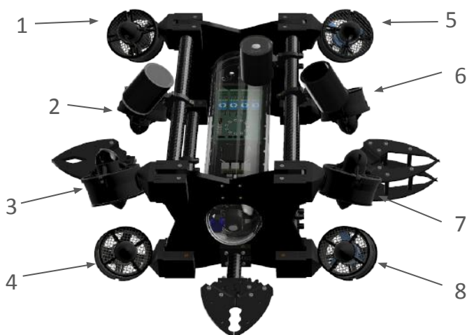
Figure 26: Dark Shark V2 thruster configuration, rendered by Mark Zagha.
