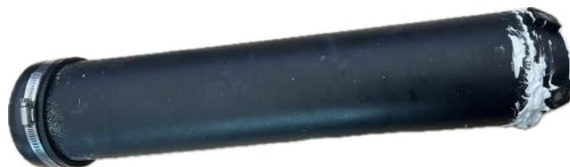
Figure 32: Night Owls' buoyancy engine, photo by Ava Palazzolo.
