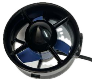
Figure 30: T200 thruster used from last years craft due to their success from last year and to save costs, photo by Isabella Wong.
