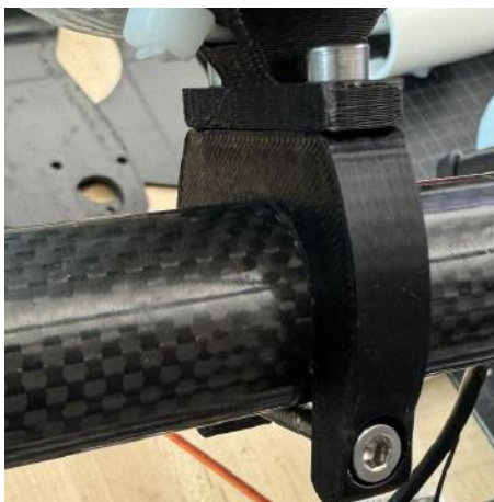
Figure 13: 3D printed clip on ROV, photo by Joshua Silversten.
