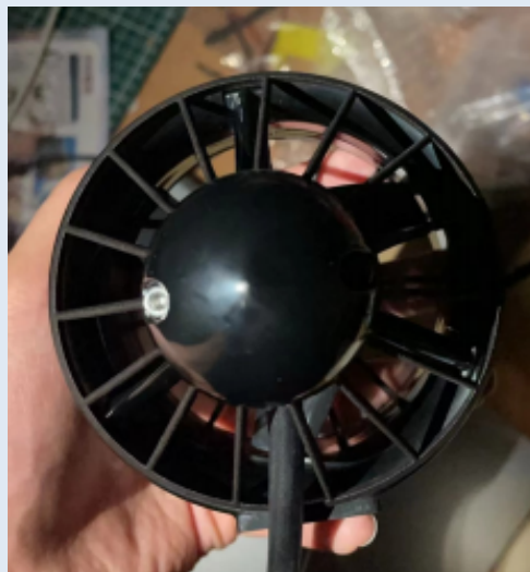
All thrusters are properly shrouded as shown
