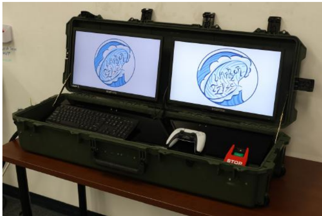
Figure 12: Topside station set up with co-pilot on the left side and pilot on the right side Taken by Jonathan Lim
