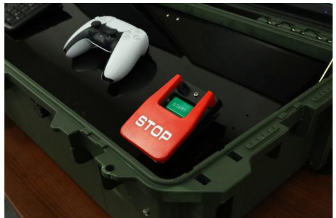
Figure 24: Emergency stop button Taken by Jonathan Lim
