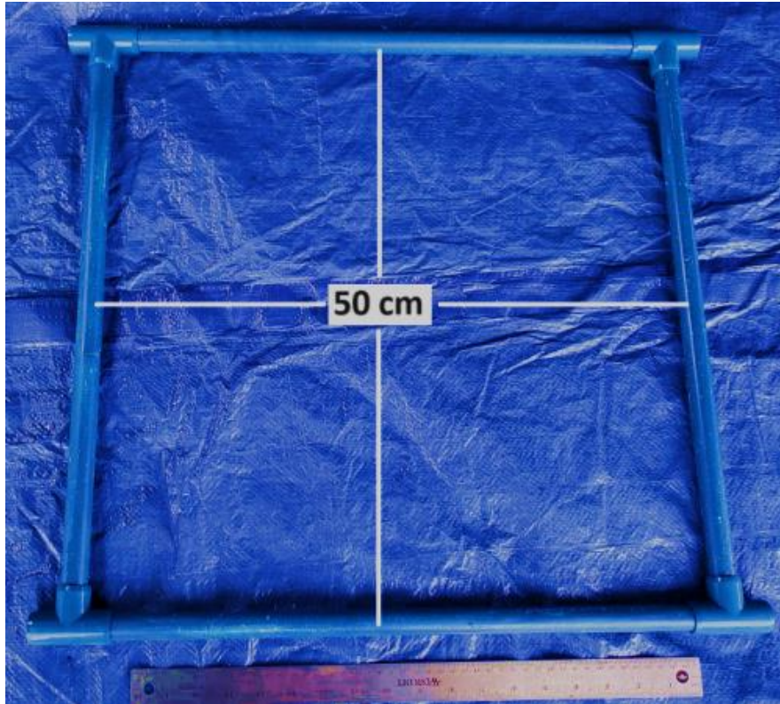
The SMART Cable designated area is a square constructed from PVC pipe painted blue.
