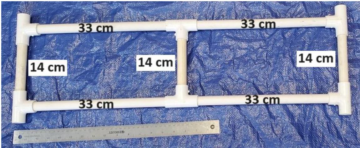
The framework of the coral restoration area is constructed from ½-inch PVC pipe.
