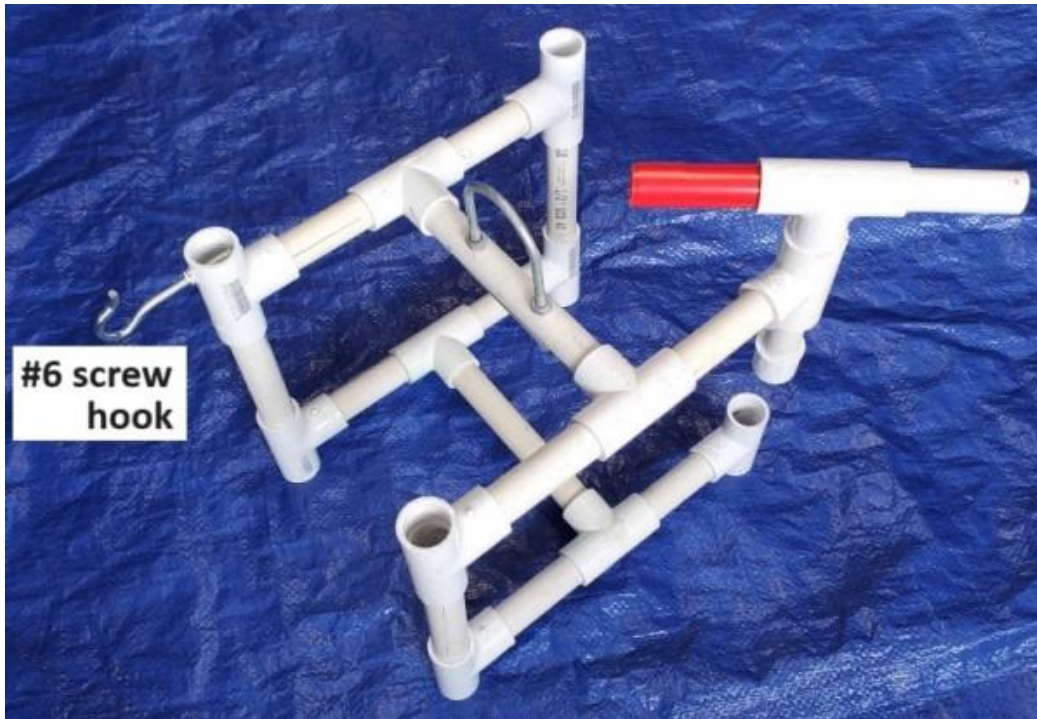
The irrigation system with the handle inserted through the \frac{3}{4} -inch by \frac{1}{2} -inch PVC tee.
