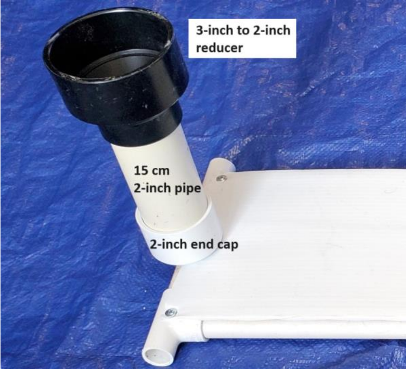
The transplant location for the branching coral is constructed from 15 cm of 2-inch PVC pipe inserted into a 2-inch end cap with a 3-inch to 2-inch reducer attached to the top.
