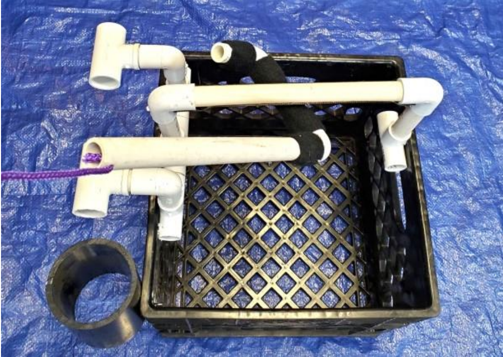
The recovery line attached to the 1/2-inch PVC pipe bale on the multi-function node.
