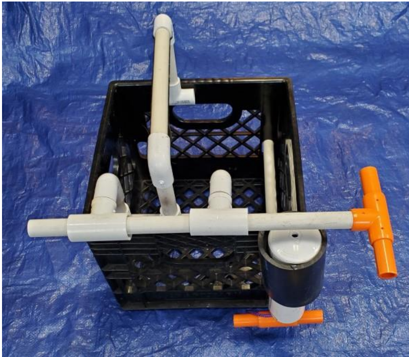
The multi-function node with the acoustic release pin holding the recovery float in place.
