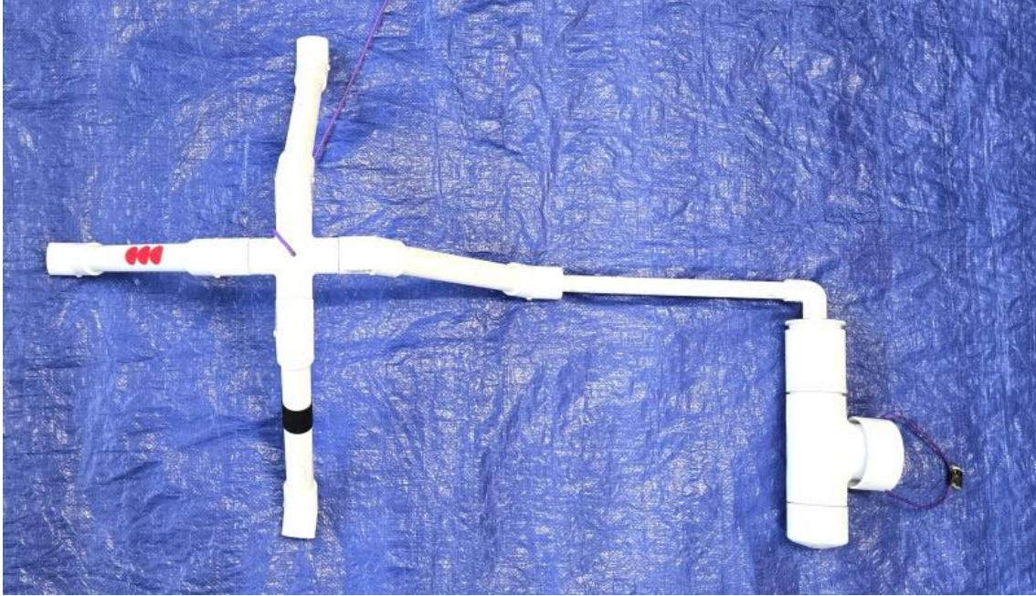
The wind farm sub-surface structure. 30 cm of ½-inch PVC pipe connects the sub-surface structure to the connection port for the offshore solar panel array.
