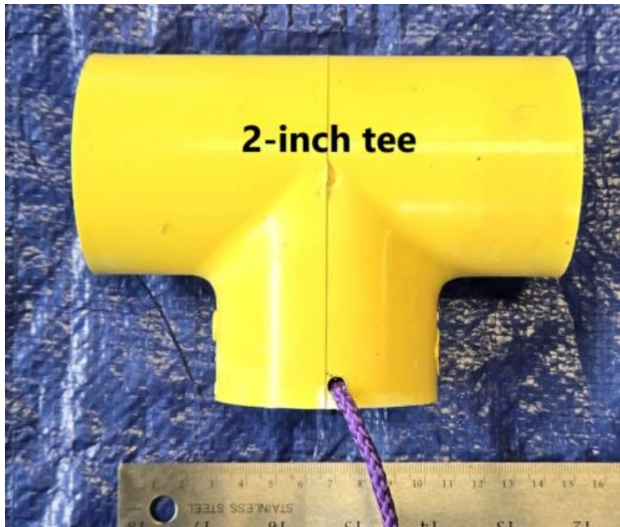
The Spotter buoy is constructed from a 2-inch tee and filled with foam flotation. A length of rope connects the buoy to the base on the bottom of the pool.
