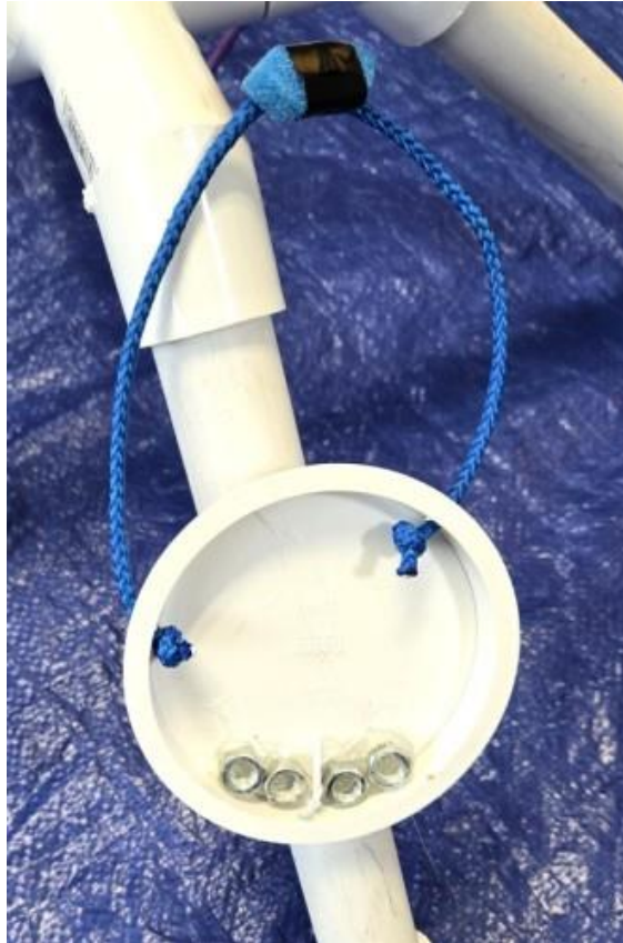
The sacrificial anode on the subsurface structure of the offshore wind turbine.
