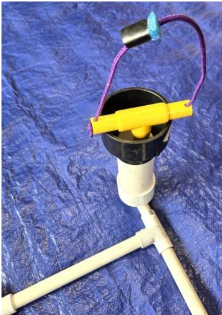
The pCO 2 connector installed into the base of the Spotter buoy.
