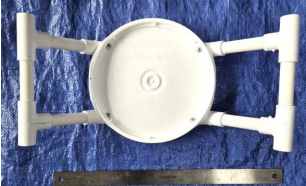
Left: A 2-gallon bucket lid is screwed onto the framework to complete the dinner platter.
