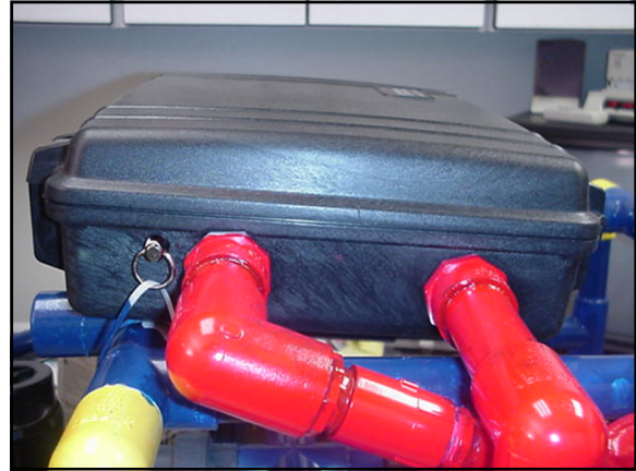
Custom made fittings to bring electrical wires to the Pelican Case from pvc frame
