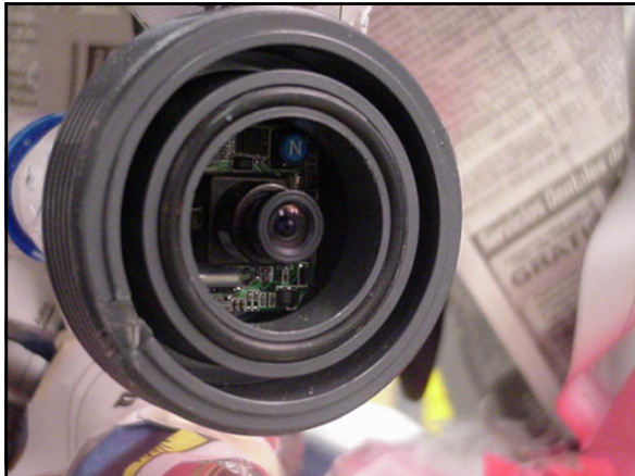
Color CCD camera housed in 1/2 a pvc union. O-ring seal visible with lexan cover off.
